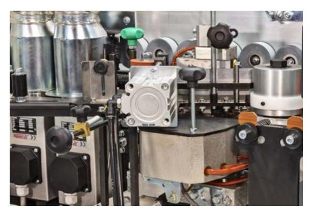
Pneumatic shear, pressure rollers, edge feeding system
